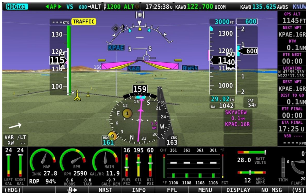
Figure 69: SkyView HDX Synthetic Vision Traffic Alert
