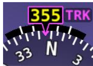
Figure 41: GPS Track substitute for Magnetic Heading indicator
