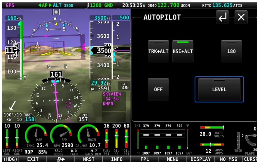
Figure 224: HSI+ALT Mode is engaged.
