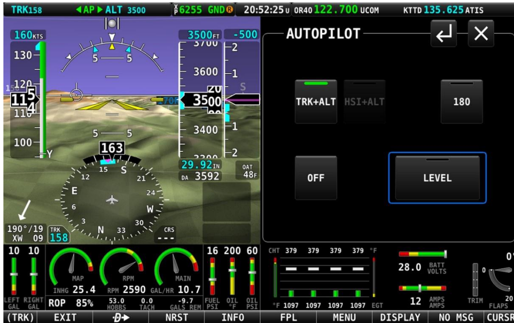
Figure 223: TRK+ALT mode is engaged.
