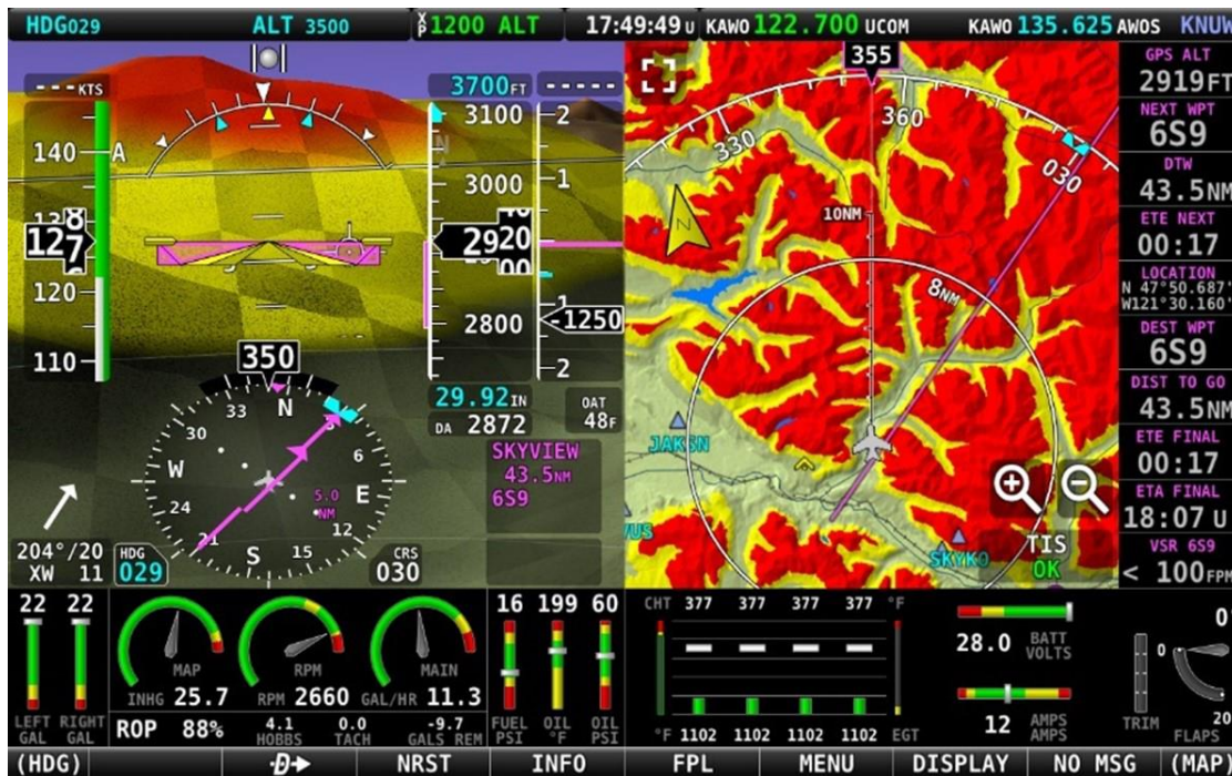
Figure 65: SkyView HDX Synthetic Vision – Terrain Alert
