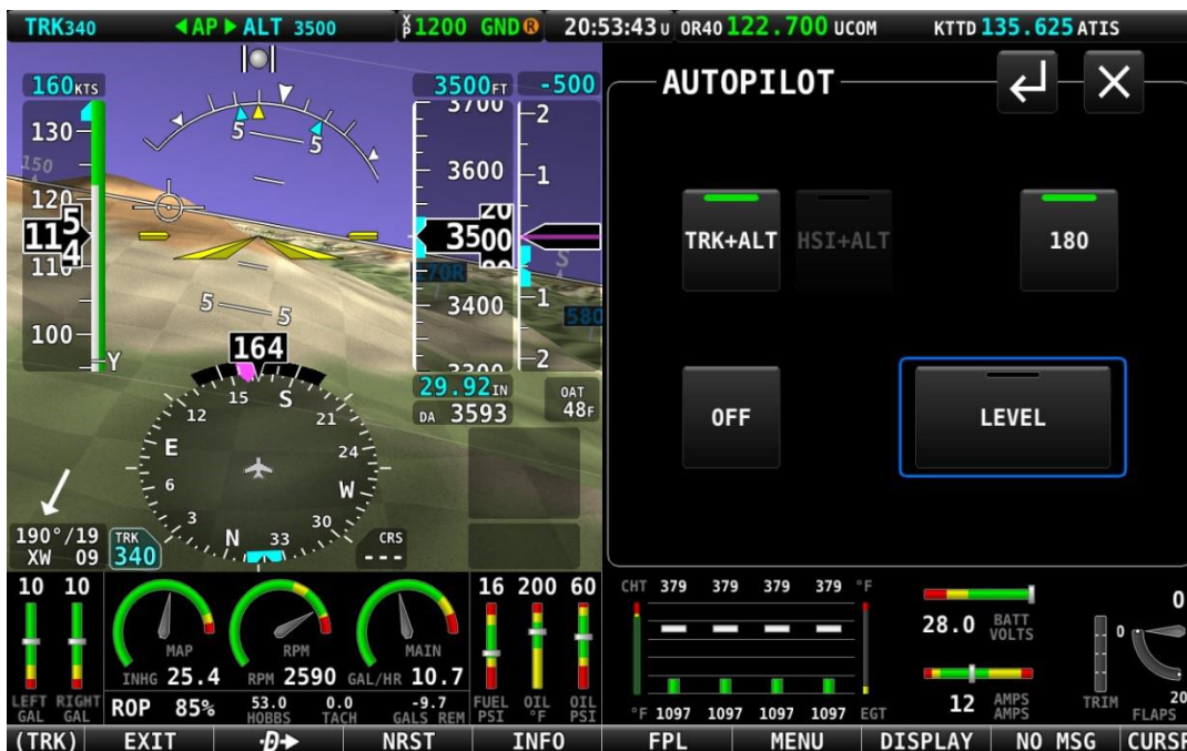
Figure 225: 180° Mode is engaged; turn is not yet complete.
