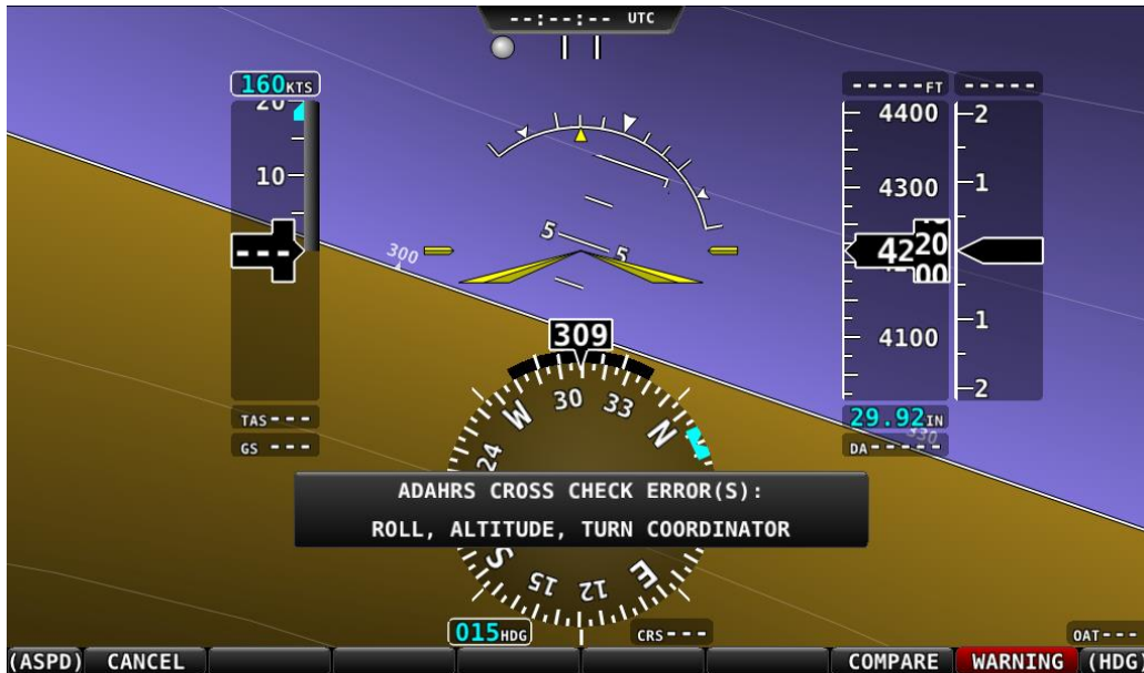
Figure 87: ADAHRS cross-checking disagreement.
