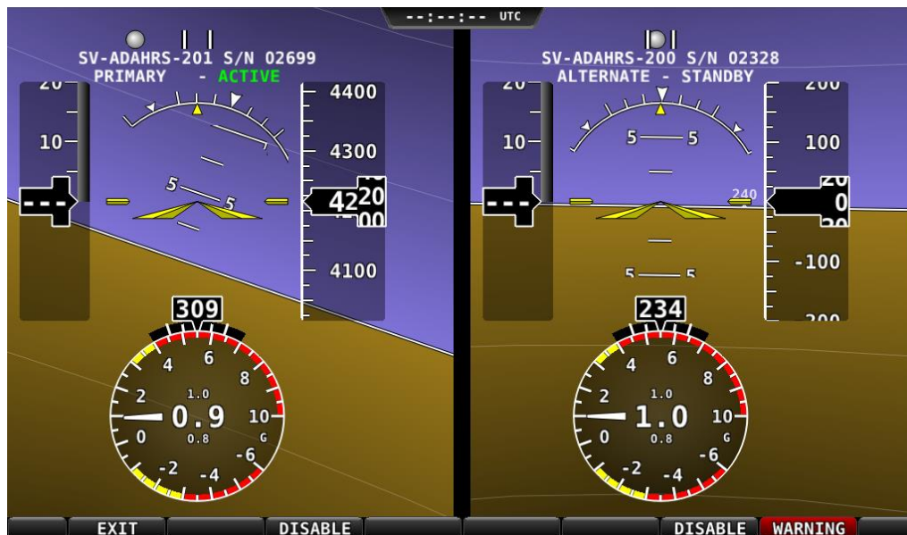
Figure 88 – ADAHRS Cross-Check Comparison (EFIS Presentation)
