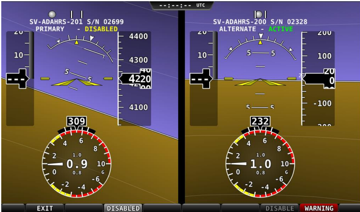
Figure 89: ADAHRS cross-check comparison (one ADAHRS disabled).
