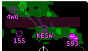
Figure 174: Missing NEXRAD data blocks.
