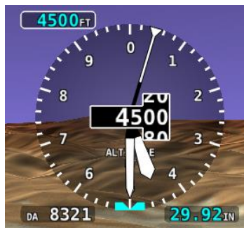
Figure 78: New Instrument Altitude Gauge
