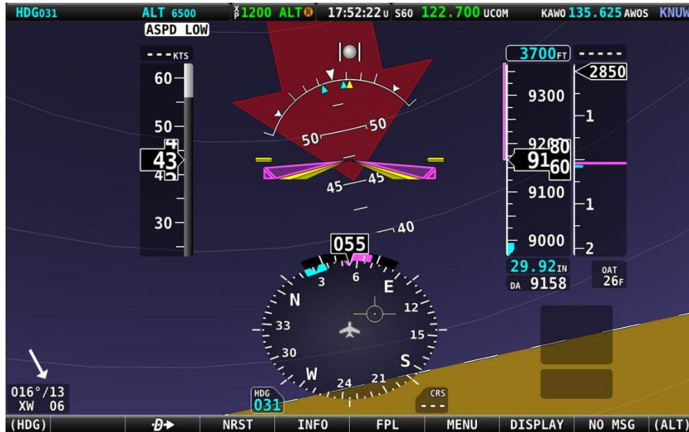
Figure 74: Extreme Pitch warning indicator arrows
