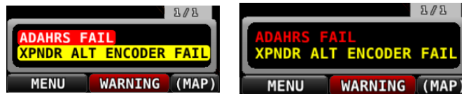
Figure 251: Unacknowledged (left) and Acknowledged (right) alerts
