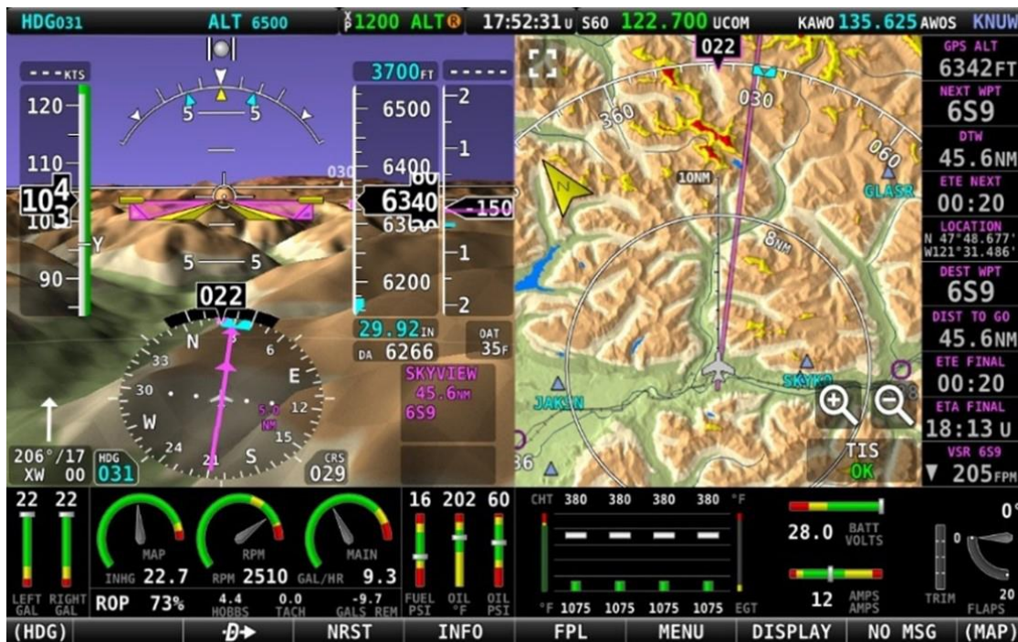
Figure 64: SkyView HDX Synthetic Vision – Normal View
