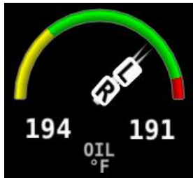
Figure 197: Examples of combined Oil Temperature widgets.
