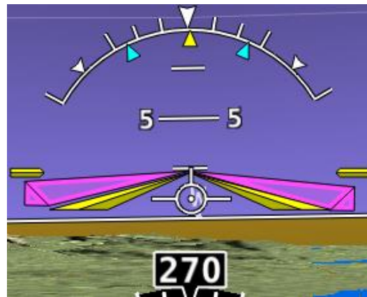
Figure 232: Single Cue / Inverted-V with Autopilot servos not engaged.
