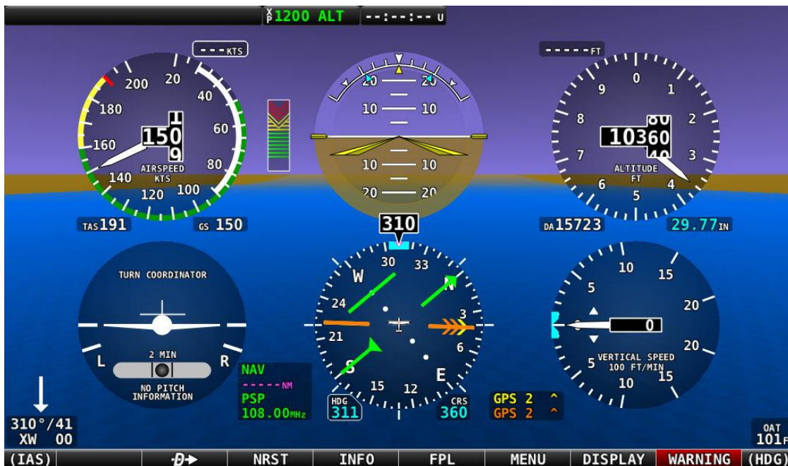
Figure 76: Six Pack PFD presentation, Synthetic Vision enabled.
