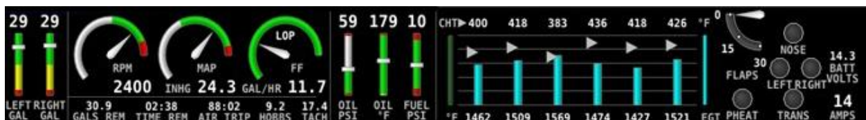
Figure 194: Example of an ENGINE BOTTOM BAND Page layout for single-engine monitoring.
