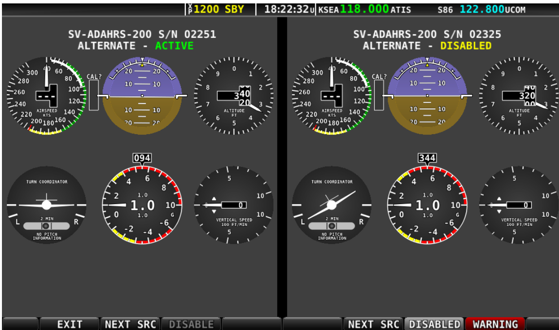
Figure 90: ADAHRS cross-check comparison (Six Pack presentation).
