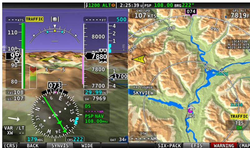
Figure 42 – SkyView Synthetic Vision Normal View
