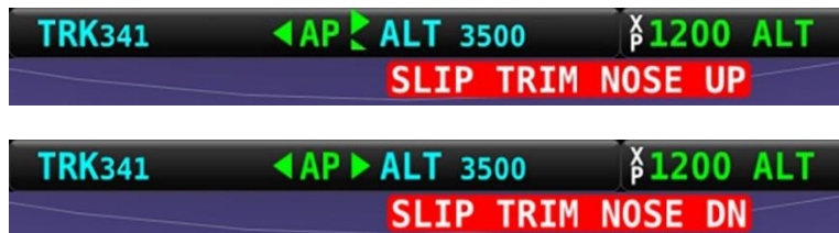
Figure 181 – Pitch Slip Trim Nose Up and Down Alerts
