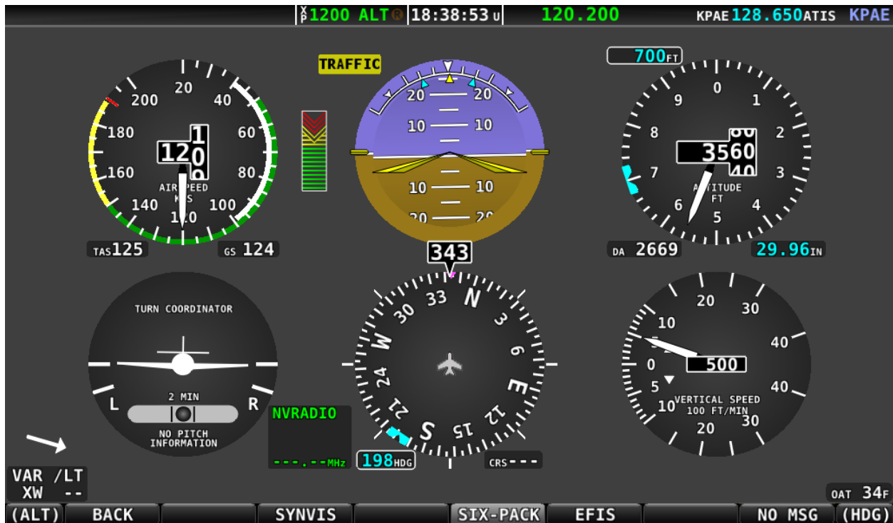
Figure 52 – Analog PFD without Synthetic Vision
