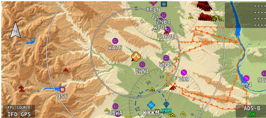
Figure 165 – Example of a PIREP Indication on Map
