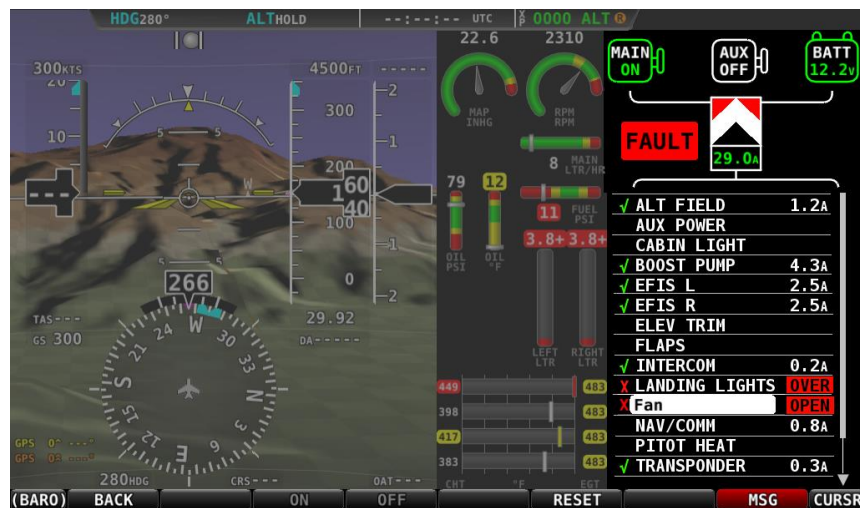
Figure 78 – VP-X Page with Fault
