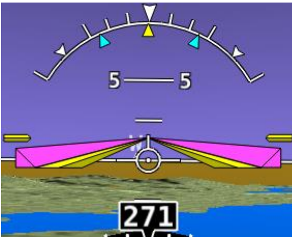
Figure 211 – Single Cue / Inverted-V with Autopilot Servos Engaged
