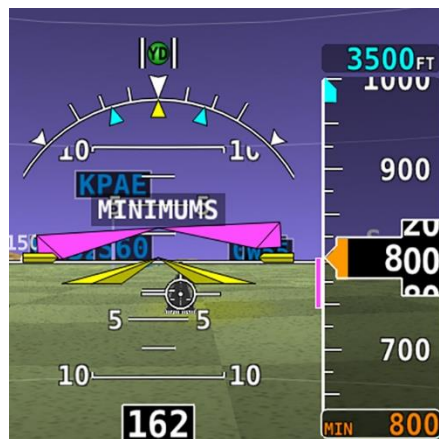
Figure 19 – MIN Bug and “MINIMUMS” Alert
