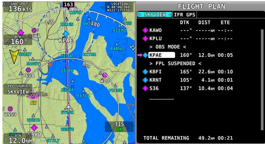
Figure 143 – OBS Mode Activated
