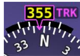
Figure 22 – GPS Track substitute for Magnetic Heading
