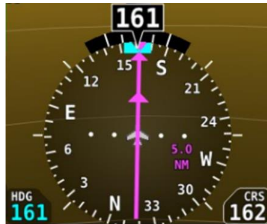
Figure 24 – HSI Example - GPS
