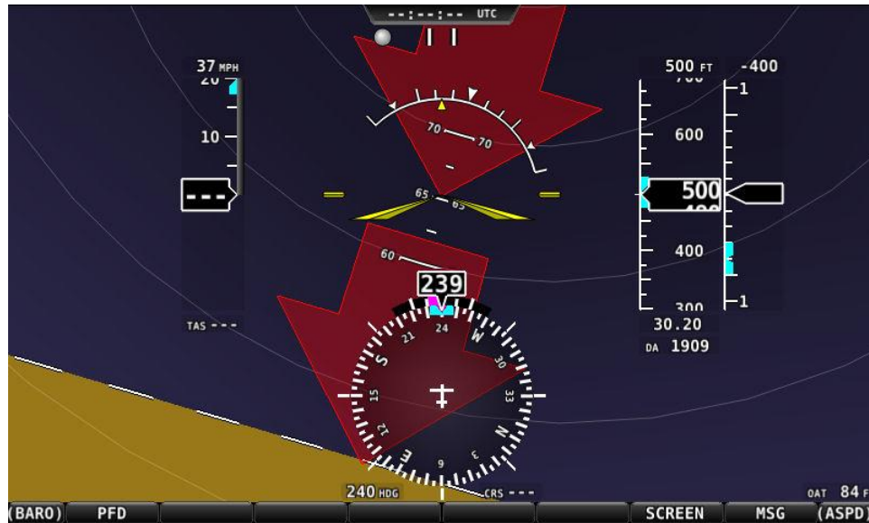
Figure 50 – Extreme Pitch Warning Indicator Arrows
