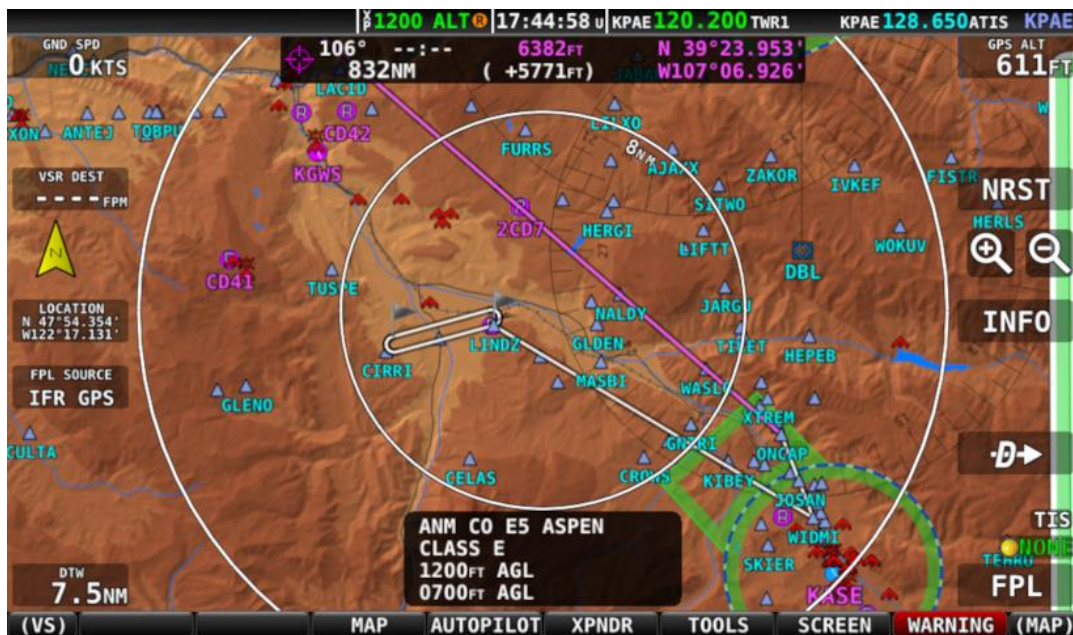
Figure 139 - Example of External Flight Plan Echo
