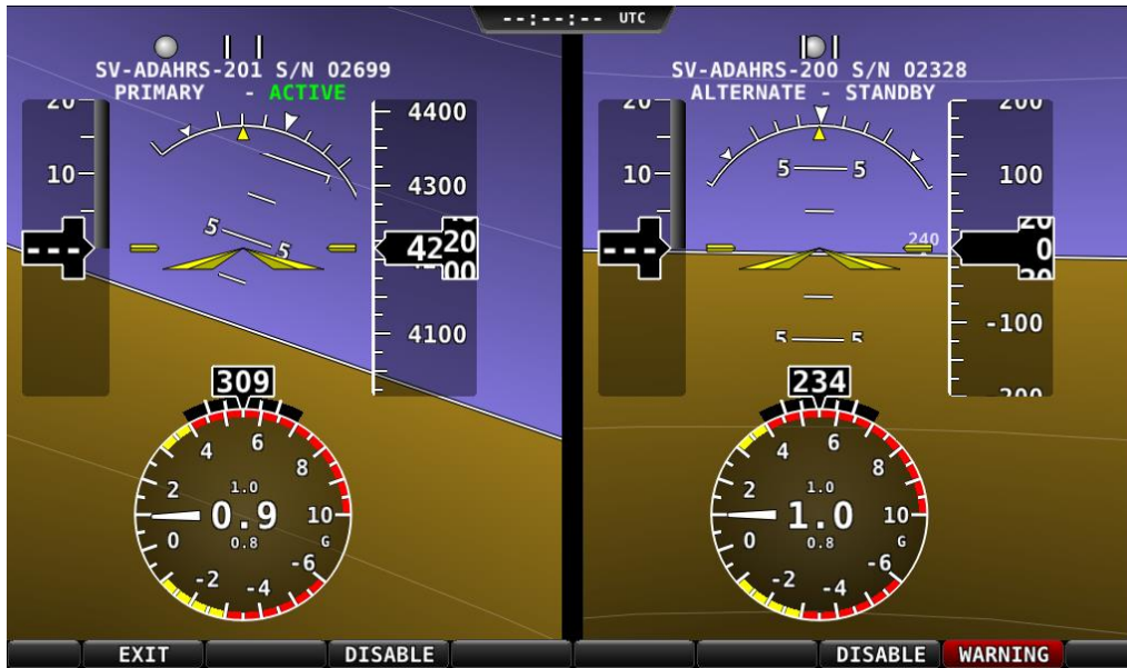
Figure 55 – ADAHRS Cross-Check Comparison
