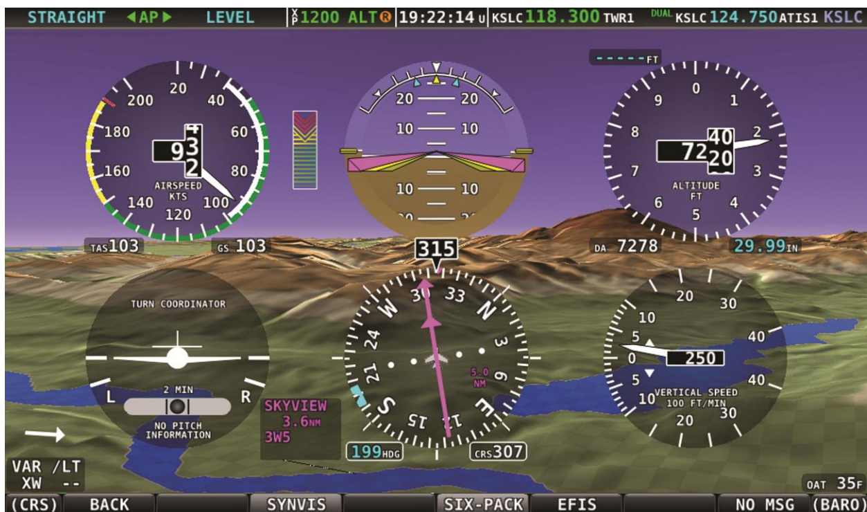
Figure 51 – Analog PFD with Synthetic Vision
