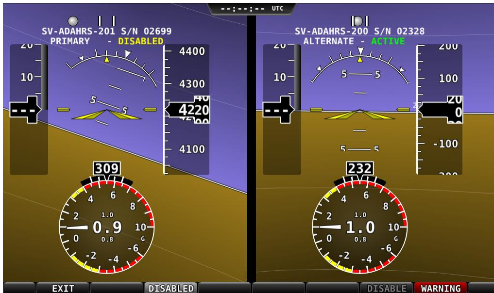
Figure 56 – ADAHRS Cross-Check Comparison (one ADAHRS disabled)
