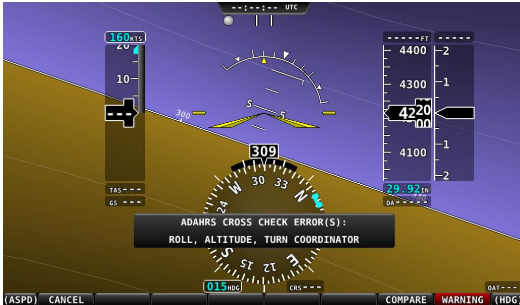
Figure 54 – ADAHRS Cross-Checking Disagreement
