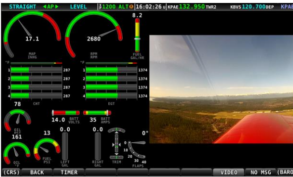
Figure 226 – Half Screen EMS/Video Display
