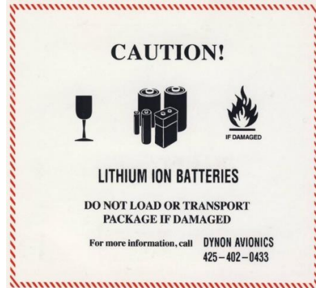
Figure 131 – Example Lithium-Ion Battery Shipping Label
