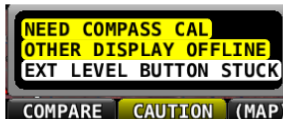
Figure 145 – EXT LEVEL BUTTON STUCK Message
