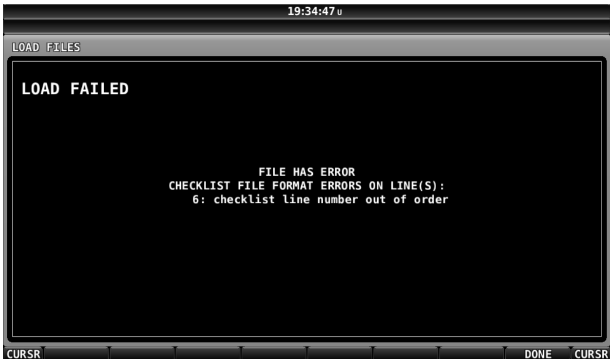
Figure 264 – Checklist File Has an Error, Line Number Displayed, Could Not Be Loaded
